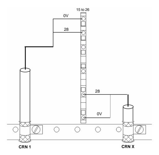
Terminals 15 - 26 manage the triggers of the various atomizers Sames, each of these twelve terminals manages two triggers, that is 24 triggers all in all. The wire 0V indicates the common and the wire 28 represents the trigger 24V.
