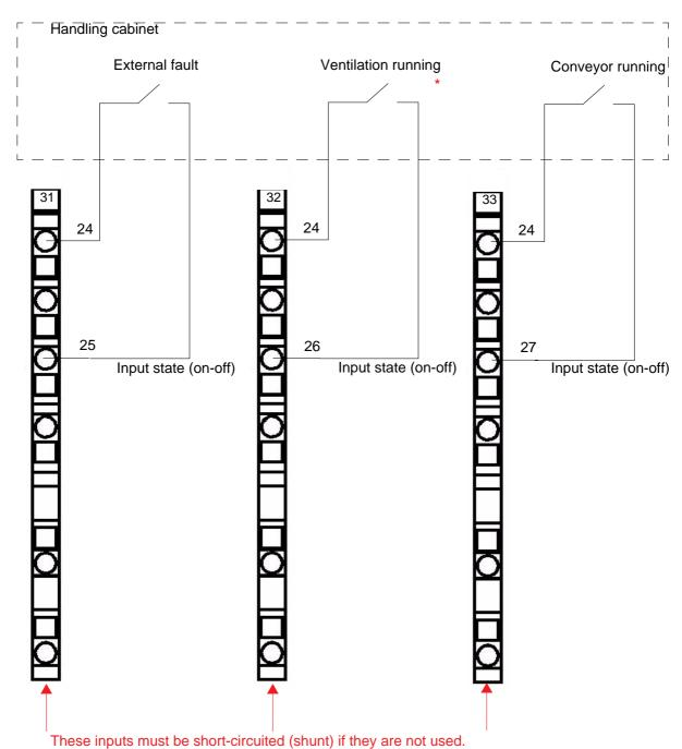
WARNING: Atomization (powder or liquid paints) must be imperatively interlocked with the operation of the booth ventilation in order to have a correct flammable or explosive limit (LEL), any other use is under the responsibility of the operator.
