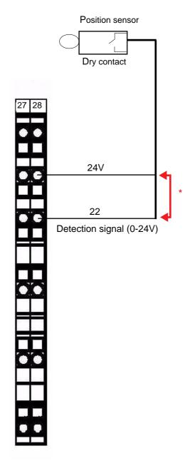
\*: bridging to be installed if detection input is not used. Except if the TCR modules are installed in the cabinet.
