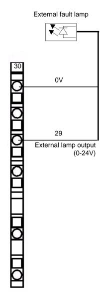
Information given by the external fault lamp (optionnal) is exactly the same as the information given by the red "Fault" indicator light located on the front face of the FCR cabinet.
