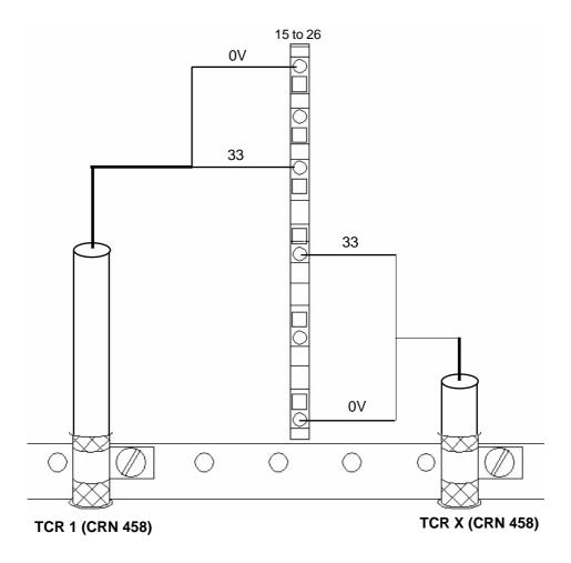
The wire 0V indicates the common and the wire 33 represents the trigger 0V.
