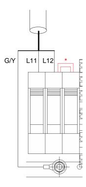
The cable recommended by Sames Technologies is 3 G 1.5 mm<sup>2</sup> (Ref.: E2CCKN004).
