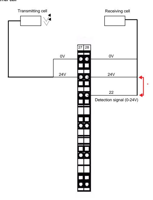
\*: bridging to be installed if detection input is not used. Except if the TCR modules are installed in the cabinet.
