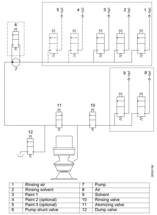
To stop atomization, switch off the pump. Then close the atomizing valve.
