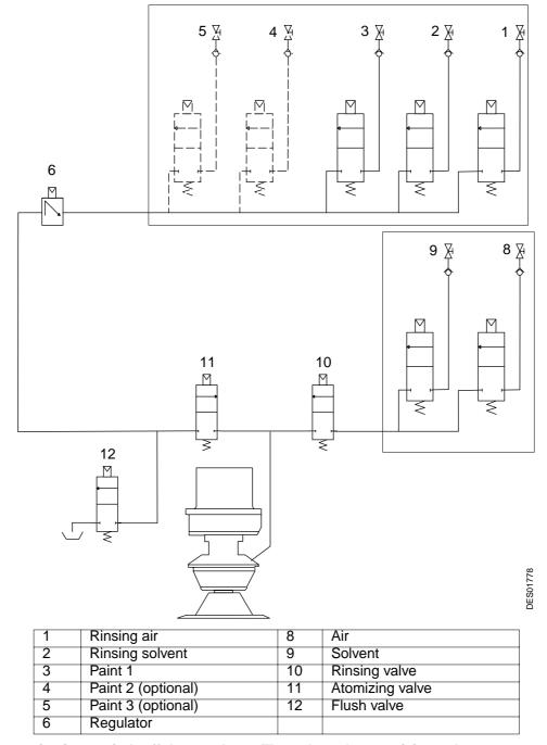
To stop atomization, switch off the regulator. Then close the atomizing valve.
