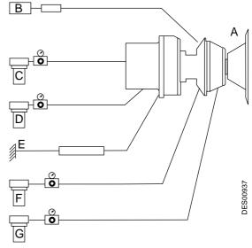
Air circuit (G) supplying the shaping air shroud is used to control stability of the paint spray.
