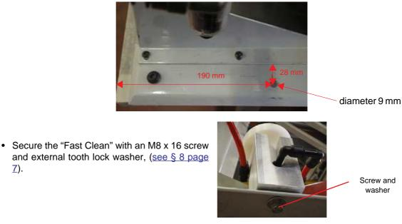
• Connect the "Fast Clean" to the cart air supply with pneumatic unions (items A and B) and hose (item 1), (see § 8 page 7).
