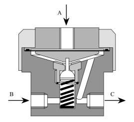
In other words, the regulator outlet pressure or regulated pressure is more or less equal to the regulator trigger air pressure. Any slight difference between these values decreases with the ratio between s/S (seat and diaphragm cross-sectional areas). Of course Pr = Pp only if Pe > Pp.
