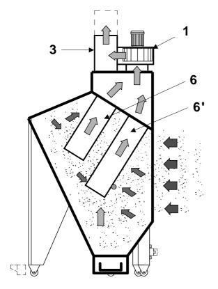
The UNIVERSAL FV 8000 module, only for use with a powder booth, permits the suction and filtering of the powder-charged air.
