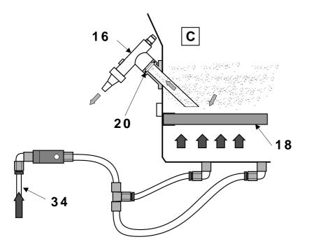
The powder released after the unclogging of the cartridges is collected in the lower part (**C**) of the cartridge holder (**B**) where it is suspended by means of air escaping through the porous bottom (**18**).
