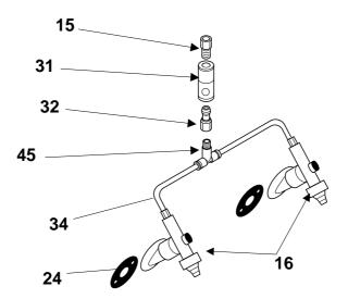
B - Pneumatic connection of the porous bottom
