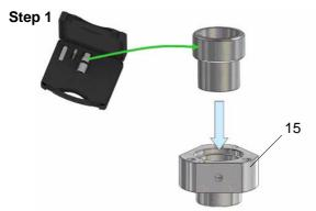
Put in place the tool on the bracket (15).
