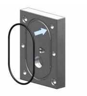
Place a new o-ring on the rear plate.
