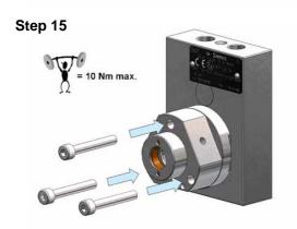
Screw the sealing system on the body (tightening torque: 10N.m).
