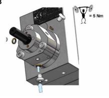
Put in place screws and washers, screw with a tightening torque 5N.m.
