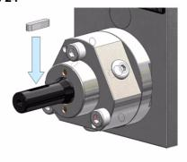
Insert the key into the drive shaft.
