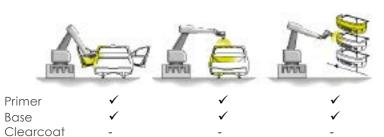
**ACCUBELL®** system is improving again performances and efficiency to a class-leading level for water based paint application with internal charge.
